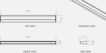
Option 1: No Dimming Number of circuits: 2 Uplight: 4000k\* Downlight: 4000k\*
