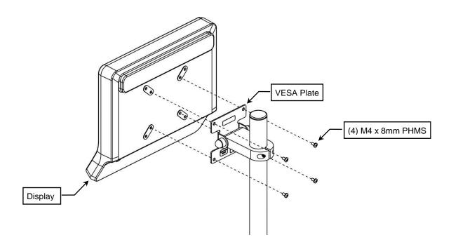
2. Adjust the height of the Display by loosening the Clamping Screw using a 3/16" Hex Wrench (provided) and moving the Display vertically along the Post. When at desired height, tighten the Clamping Screw until the Display is secured in place.
