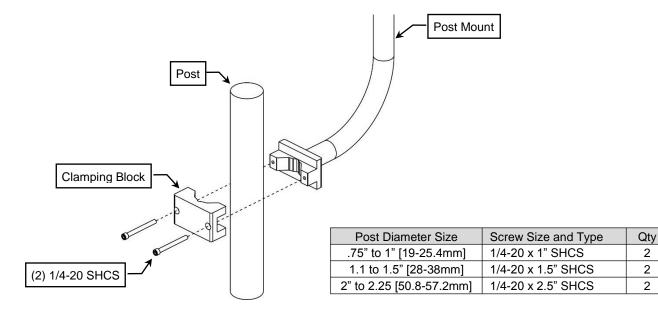
3. Adjust the height of Clamping Blocks on Post to allow enough clearance for Post Mount Display.
