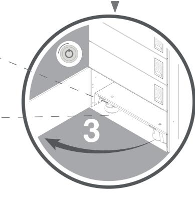
Unlock/Open the lowest cabinet door using the Service Key to access the footmaster wheel set.
