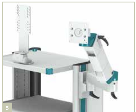
Variable height support arms (with or without a swivel arm) can be attached by means of a bottom shelf, or else fastened directly to the power column.
